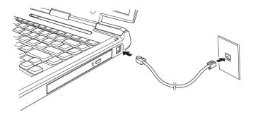
Figure 4-11 Connecting the internal modem
